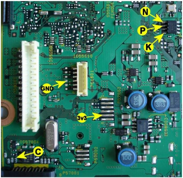
Stick the logic board with some double-sided tape onto the mainboard, and connect wires from points C, P, N, K, GND and +3v3 to the corresponding points on the Logic Board.
