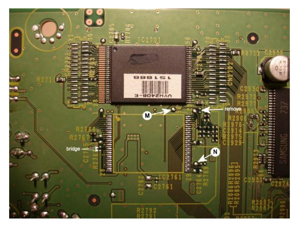
Install the supplied Flash chip at the empty spot on the board (IC2761). Make sure you align the chip correctly; pin 1 is indicated with a dot on the chip.
