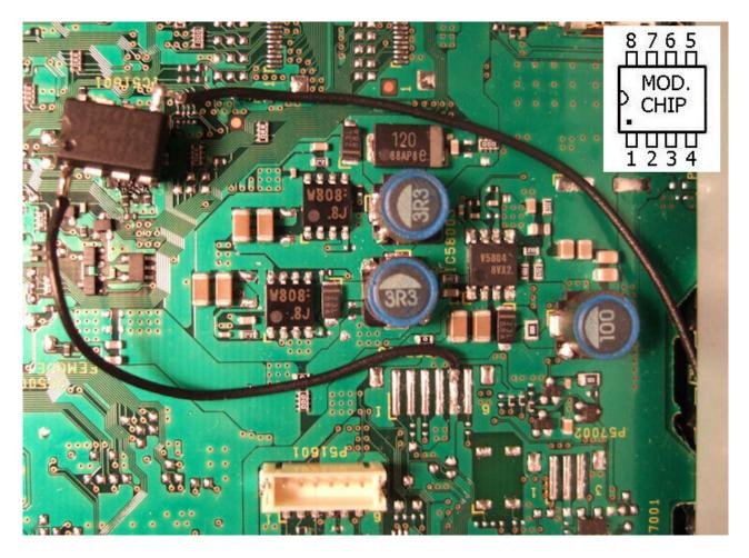
If you're not confident with the "piggy-back" fitting method just use wires to connect all 6 pins of the mod. chip.
