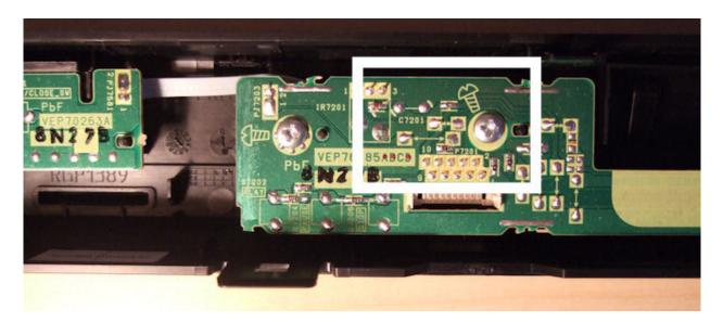
Connect pin #5 to the point on the front panel PCB shown below.
