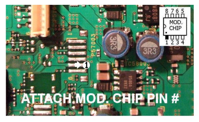
Mod. chip pins #2, #3, #4 and #8 should be connected to the small 8 pin chip as shown.
