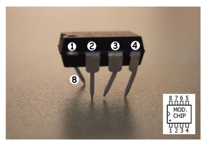
Bend the pins into position and then hold it against the chip on the board to make sure they are lined up correctly. Once all the pins are lined up solder pin #8 first, then you can carefully position the mod. chip by rotating it slightly and solder pins #2, #3 and #4. It should then look similar to the image below.
