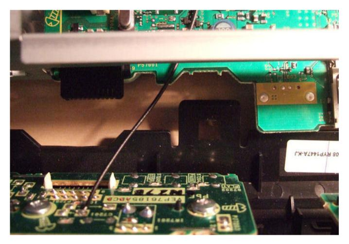
When re-fitting the front panel check that all 7 plastic clips are fully in place, otherwise the electrical connectors may not contact correctly.
