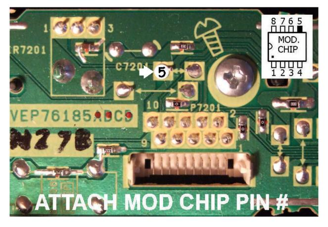
Bring the wire for mod. chip pin #5 in under the metal plate at the front of the player, ensuring that it doesn't block the connector shown at the left side.
